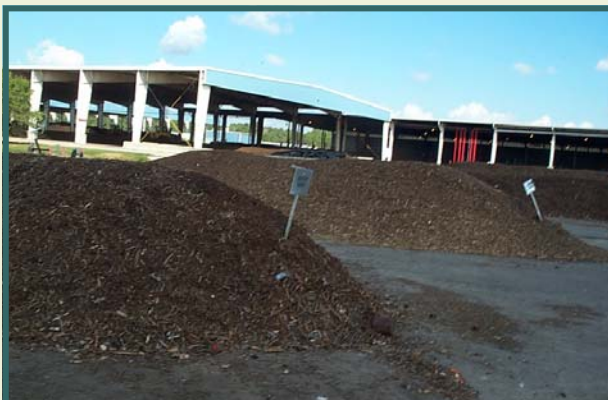
Pilot windrows comprised of food and yard waste at Disney's Reedy Creek
