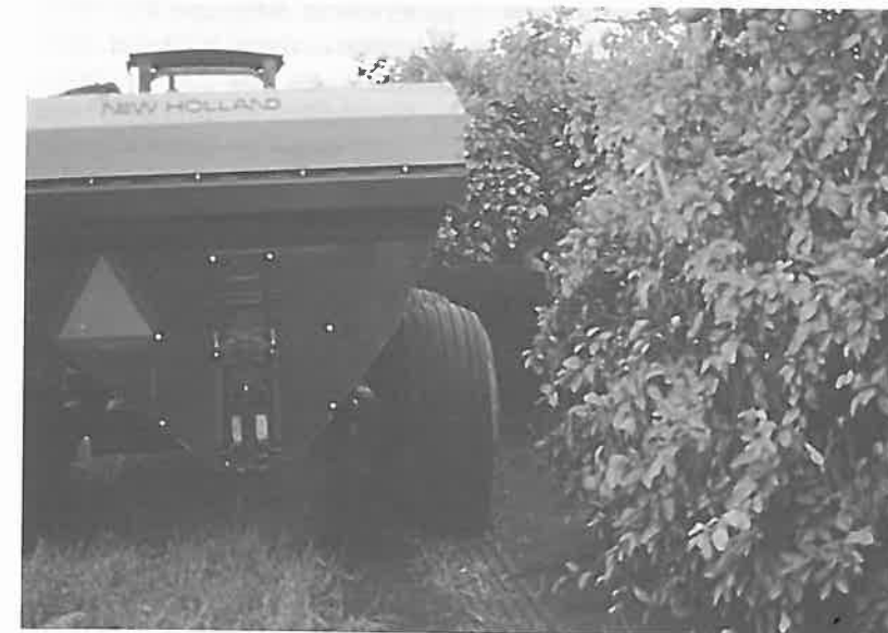
Figure 9-2. Composted municipal waste (CMW) is applied to bearing citrus trees with a New Holland 3000 side-discharge spreader as a 5–10cm thick mulch layer within the row to cover about 80% of the root system. The rate at this location ranges from 150–170 metric tons per hectare of treated soil area.
