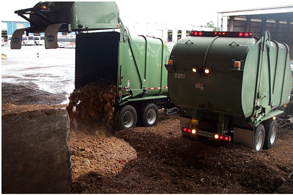
Food Waste Discharged onto Bed of Yard Trash
