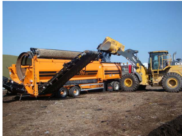
Loader deposits compost into hopper.
