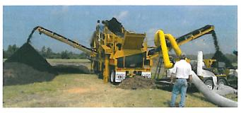
The Redox equipment consists of a feed hopper supplying material to a pair of deck screens, and also employs a built-in air separation unit. Separated fines are discharged from the rear of the unit and overs are removed via a small side conveyor. The removed plastics component can be fed directly into a roll-off container or can be discharged on the ground.
