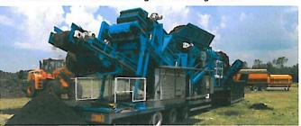
The Wind Sifter is a separate attachment that mounts directly above the overs conveyor of the Doppstadt 720 Trommel and is powered via auxiliary hydraulics on the trommel. The unit consists of a fan with flail blades, which create a vacuum drawing plastic out of the overs and discharges them through a 14 inch flexible hose.
